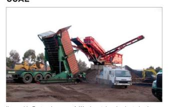
Ibercoal in Portugal uses an A-Ward container loader to load coal into shipping containers for export.
