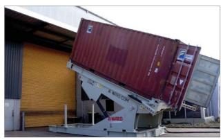
The world's largest clay ore mines use A-Ward container unloaders to unload ball bearings to grind down coarse clay material.
