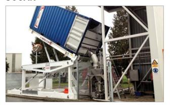
Malayan Sugar Manufacturing Co uses an A-Ward container loader to load containers for Heinz Wattie's. Heinz Wattie's uses an A-Ward container unloader to unload sugar for jam manufacturing.
